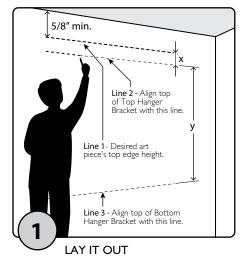
Lay out the Móz Weave Art top edge on the wall, Line 1, leveled and at the desired height (you'll need at least a 5/8" clearance above the top edge of the art piece). Then lay out Lines 2 and 3 below—where the top of the Hanger Brackets will align—using the "x" and "y" dimensions included with your art piece.
