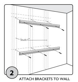
Attach Top and Bottom Hanger Brackets to wall studs with screws following your layout. Shift Hanger Brackets from side to side to line up holes with studs.
