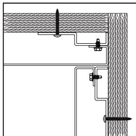
Detail showing two End Key Bars attached to plywood with two typical inner end panels attached.
