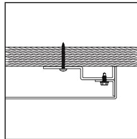
Detail showing an End Key Bar attached to plywood with one outer finished end panel attached.
