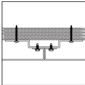
Detail showing a Mid Key Bar attached to plywood with two typical mid panels attached.
